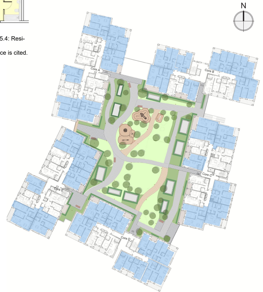
Figure 8.36 - Block 6 first floor plan with dual aspect units highlighted in blue.
