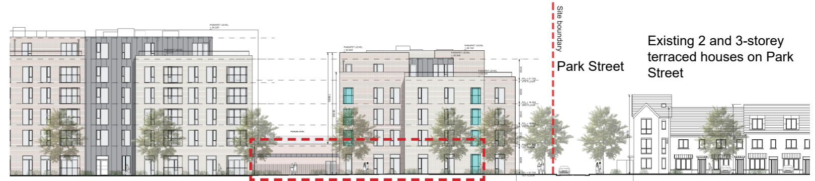
Figure 8.31 - Block 6 North Elevation on Belltree Avenue, Creche and play area outlined in Red.
