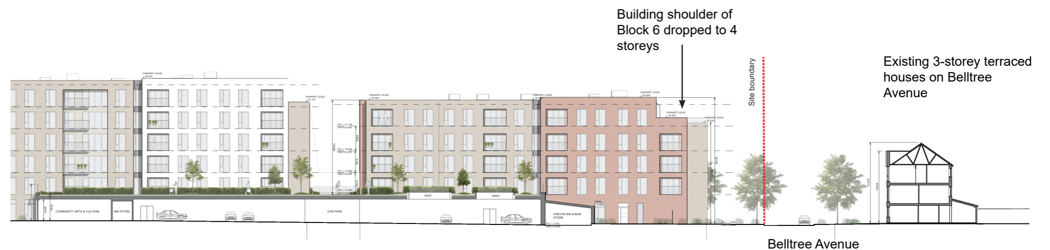
Figure 8.17 - Block 6 Section H-H showing height and massing reduction to north across Belltree Avenue
