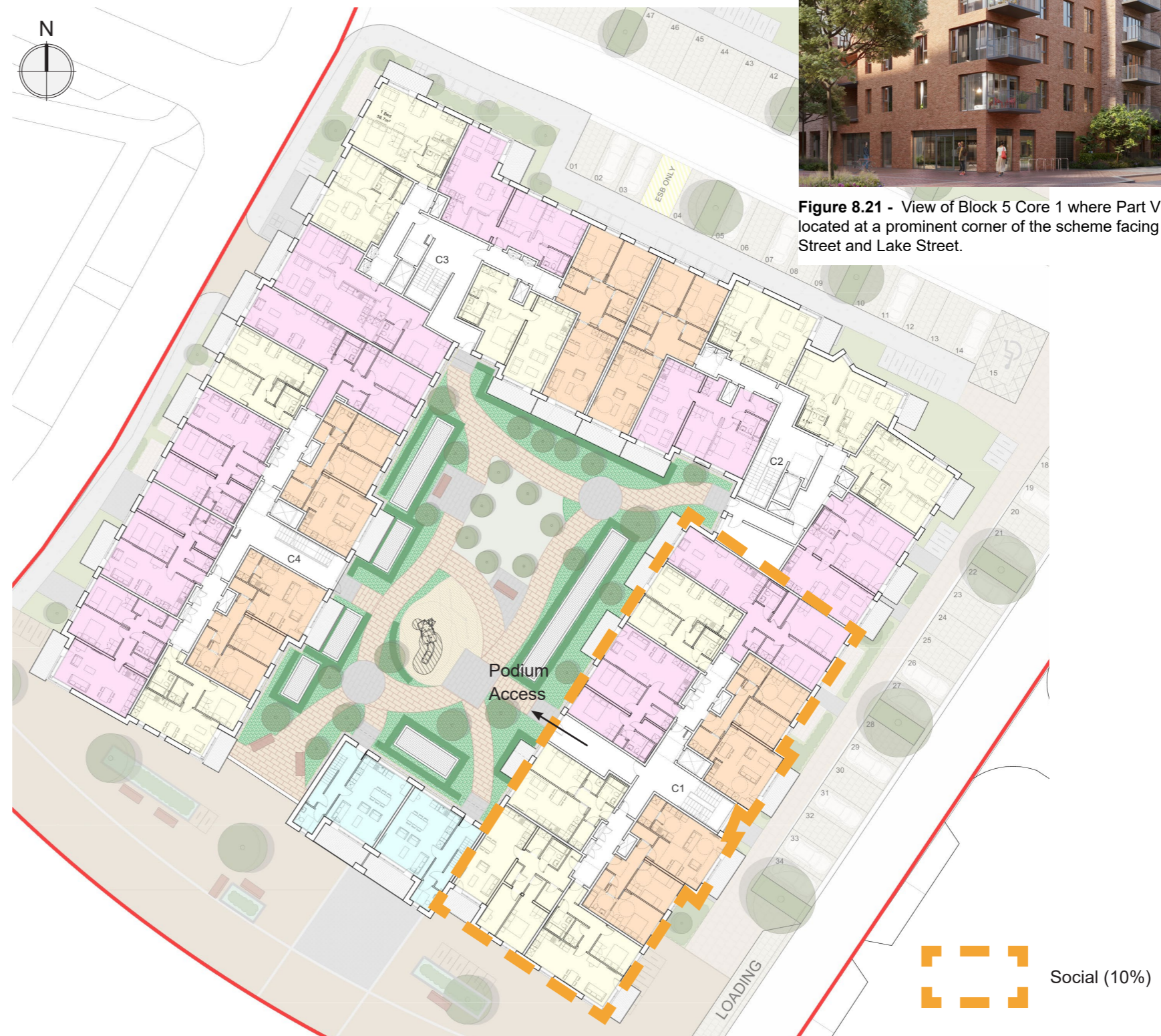
Figure 8.20 - Block 5 first floor plan with Core 1 Part V units highlighted. Part V residents have direct access to the podium level communal amenity space as well as access to the 4th floor roof terrace.
