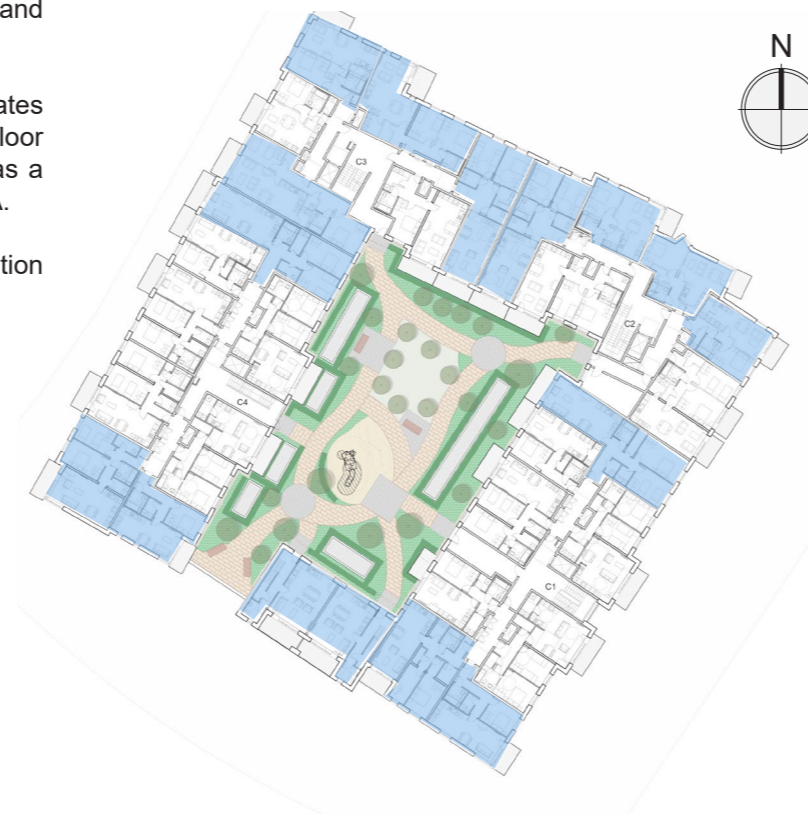
Figure 8.35 - Block 5 first floor plan with dual aspect units highlighted in blue.
