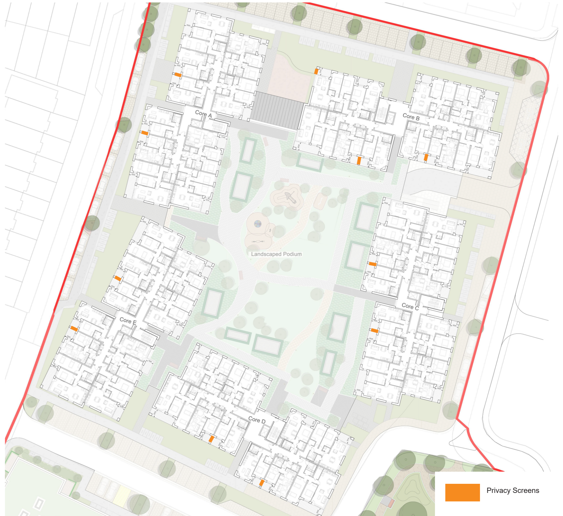
Figure 12.12 - Second Floor Plan (Typical) Location of Privacy Screens between adjacent balconies at Blocks 6
