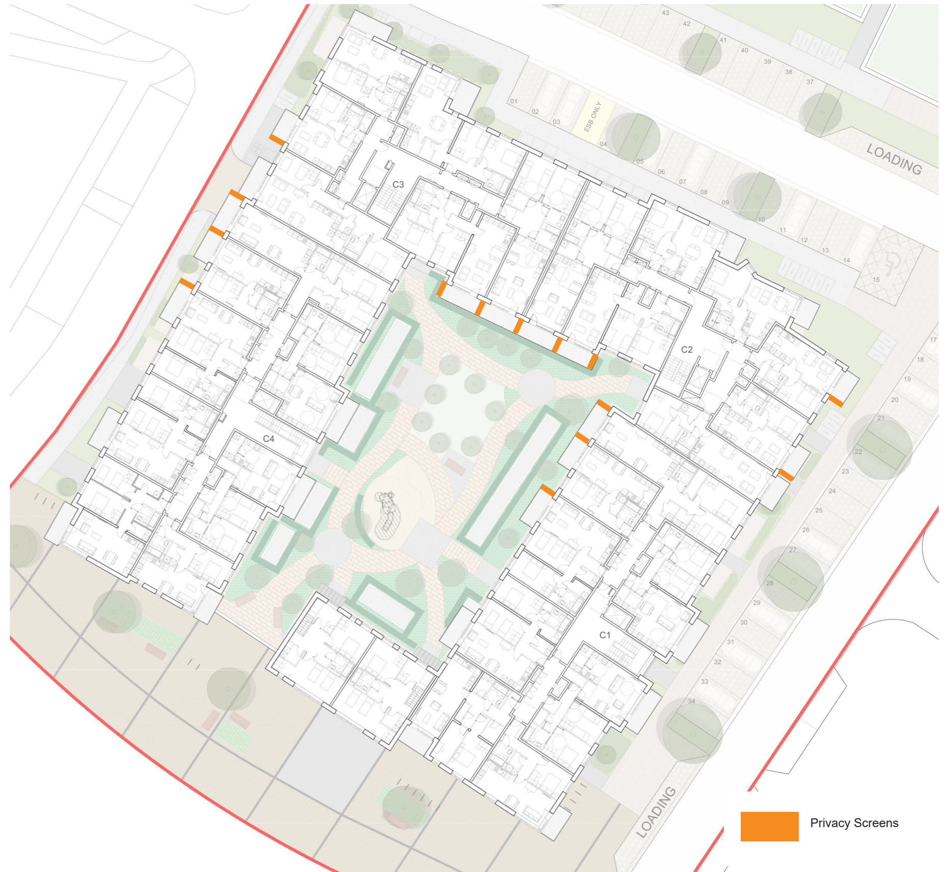
Figure 12.10 - Second Floor Plan (Typical) Location of Privacy Screens between adjacent balconies at Blocks 5
