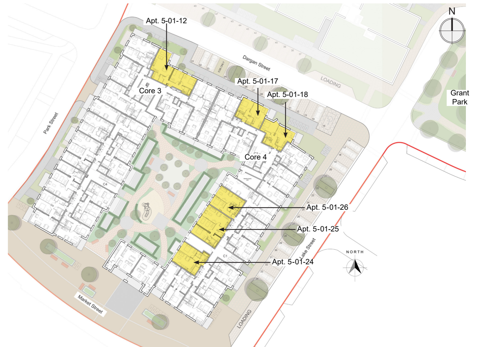
Figure A.1 - Block 5 First Floor Plan with dual aspect apartments whose primary aspect falls within 45 degrees of due north and west-north-west facing single aspect apartments facing courtyard highlighted in yellow.
