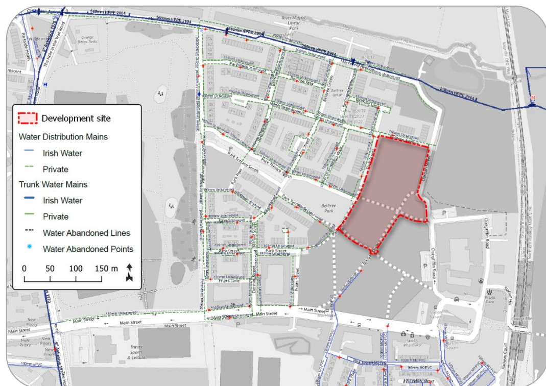
Figure 6 – Existing local water supply network (map data and imagery: Uisce Éireann, OSM Contributors)
