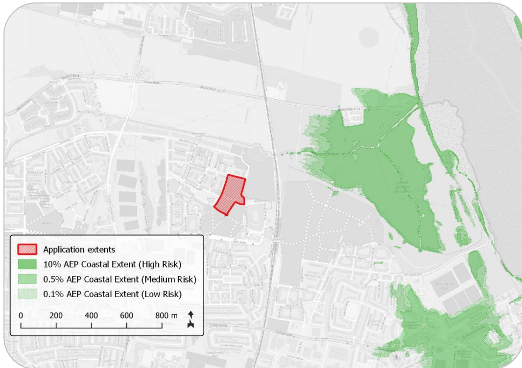
Figure 8 – FRAMS mapping of coastal (tidal) flood risk extents (sources: Office of Public Works, OSM Contributors)
