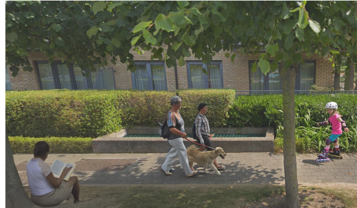
Figure 4.2 - Linear vent and shrub planting provide privacy to private terraces at Bushy Park House, Dublin.
