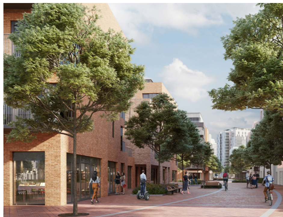
Figure 0.6 - Shared surface on Market Street with flush kerbs to signal pedestrian and cycle priority and slow traffic speeds
