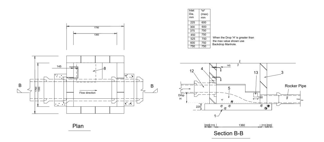
Ramp Manhole Details For Pipe Diam's. 150, 225, 300, 375, 450, 525, 600, 750mm Drop < 750mm
