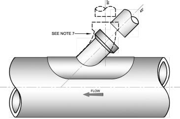
THE USE OF 90° "Y"-BRANCH OR SADDLE CONNECTIONS TO THE SEWER MAY BE ALLOWED, PROVIDED THE SADDLE OR BRANCH INCORPORATES A SWEPT TEE CONNECTION TOWARDS THE DIRECTION OF FLOW OF THE SEWER.
