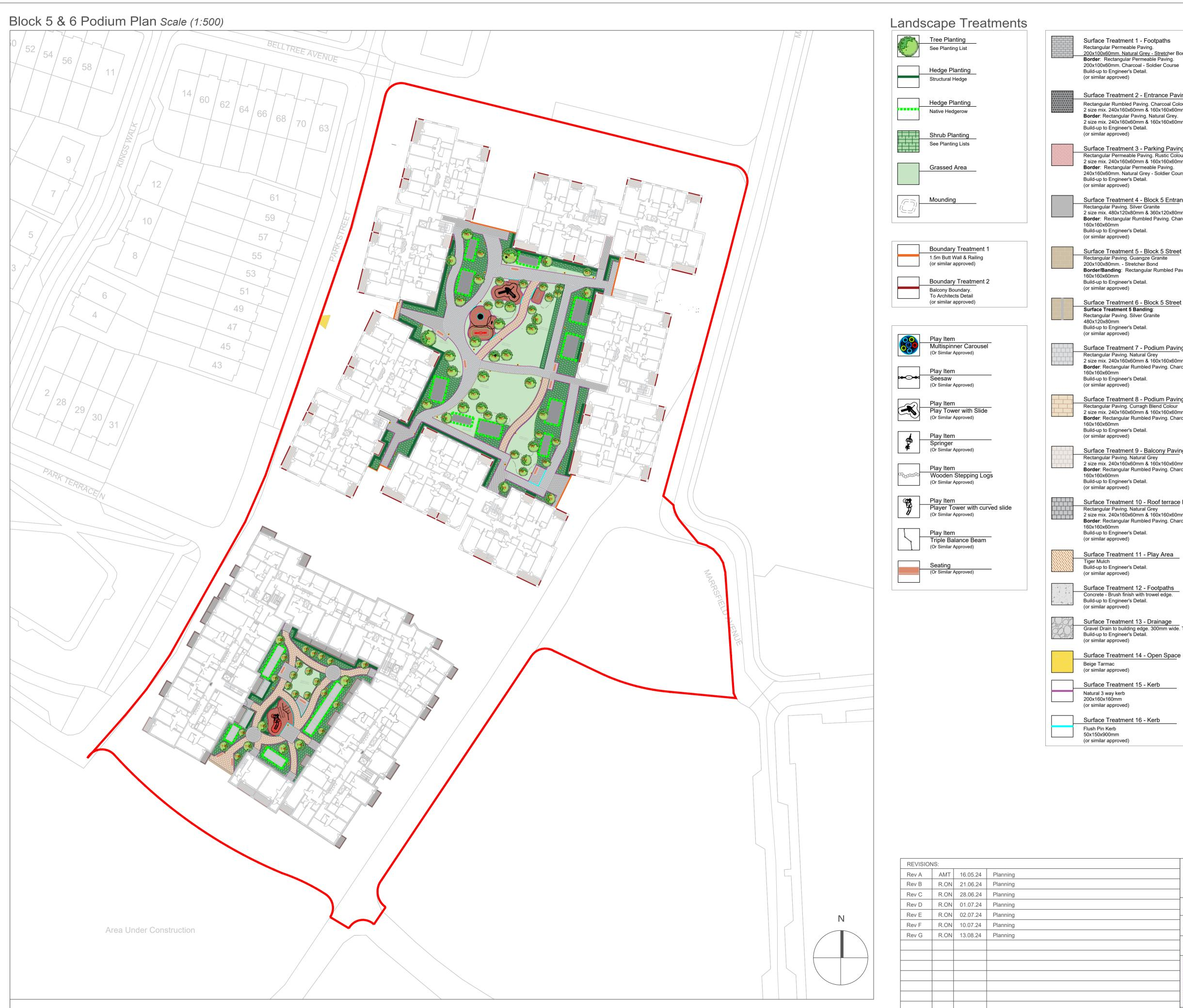
Surface Treatment 1 - Footpaths Rectangular Permeable Paving. 200x100x60mm. Natural Grey - Stretcher Bond Border: Rectangular Permeable Paving. 200x100x60mm. Charcoal - Soldier Course Surface Treatment 2 - Entrance Paving Rectangular Rumbled Paving. Charcoal Colour 2 size mix. 240x160x60mm & 160x160x60mm - Stretcher Bond Border: Rectangular Paving. Natural Grey. 2 size mix. 240x160x60mm & 160x160x60mm - Soldier Course Surface Treatment 3 - Parking Paving
